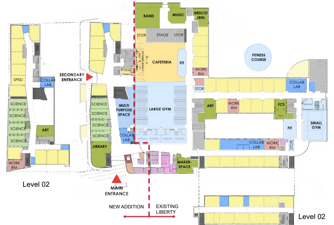
Final Floor Plans Classrooms in yellow, Collaboration spaces in blue, Workrooms in red, Specialty in green
