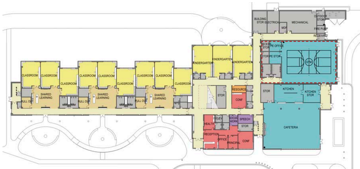
Ground floor plan with classrooms, main office, gym, cafeteria and kindergarten classrooms
